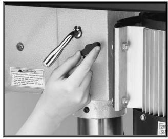
Figure 23. Loosening the lock knob.
